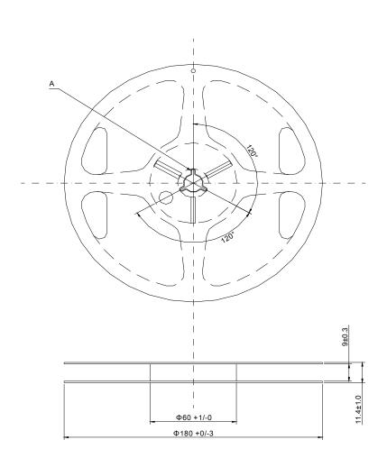
Material:Polystyrene (Conductivity) unit:mm
